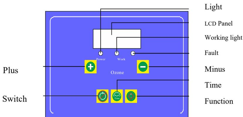
5.1.1 On/off button: In off/on state, press this button for more than 2 seconds to turn on/off when the power indicator is on;
