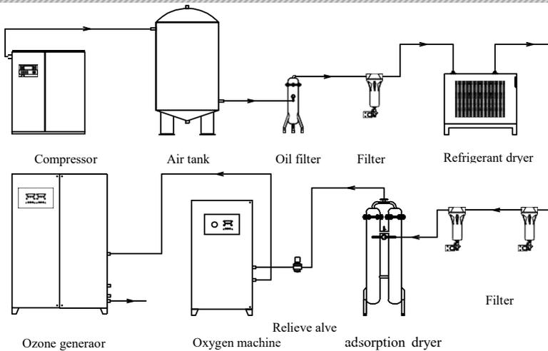
A complete ozone disinfection system is composed of 1 ozone generator, 1 oxygen generator, 1 adsorption dryer, 1 freeze dryer, 1 air compressor (air storage tank), and air filter. Processing system composition; see the picture below for the overall system composition
